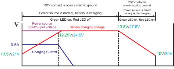
Battery Charging Voltage Curve (Red Line): Green: 12V Light Blue: 24V
